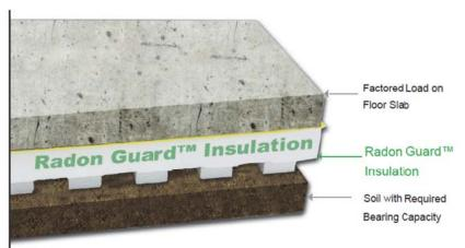
Radon Guard™ insulation¹ is a patent-pending sub-slab depressurization panel that directs soil gas movement between the ground and the air barrier system to a vent pipe. This bulletin provides guidance on recommended PlastiSpan insulation types based upon maximum specified loads.
